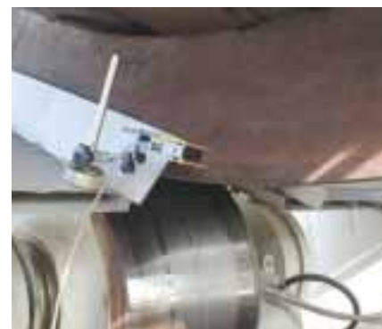
Measurement of the axial runout of the tyre.
