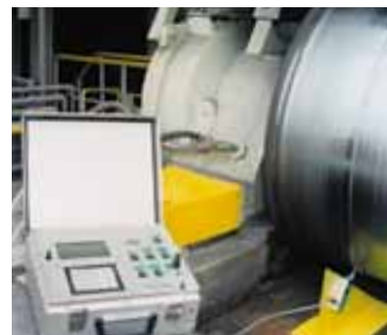
Measurement of the axial runout of the tyre.
